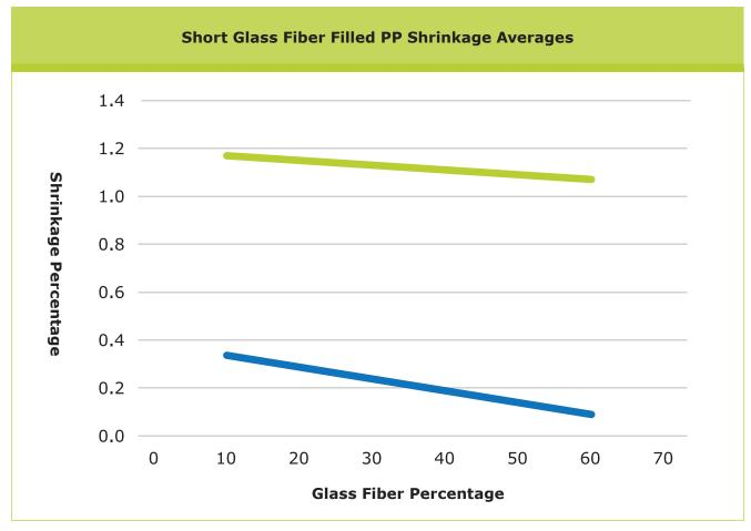
Note: Values are based on specimens with 1-3mm wall thickness.
