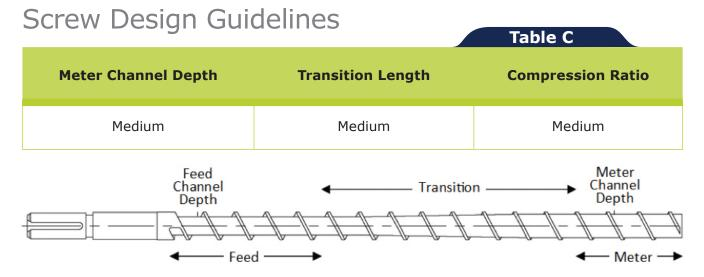
For PP formulations, including those containing short glass fiber and minerals, the suggested compression ratio should range from 2.4 - 4.0:1. The recommended compression ratio for long fiber PP should range from 1.8 - 2.5:1.
